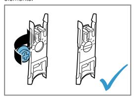
The slot in the adjustment screw must be horizontal at first.
